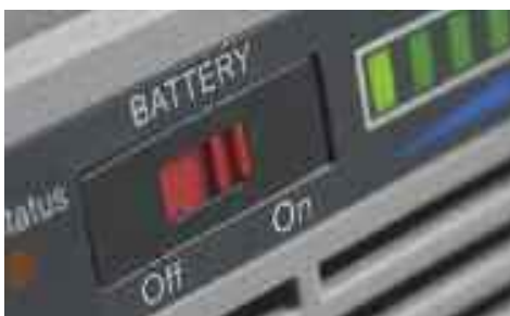
An extra control panel for the battery: ON/OFF switch, LED display showing the battery charging state
